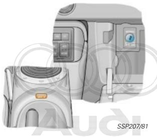
The Audi TT Coupé has a disable function for deactivating the front passenger airbag.
