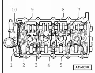
The two markings on the camshafts must be in line with the two arrows on the bearing caps -arrows-.
