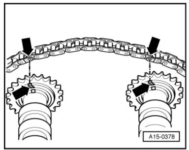
The distance between notches -A- and -B- on the camshafts must be 15 drive chain rollers. The illustration shows the exact positions of the 1st and 15th rollers on the sprockets.
