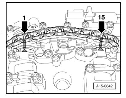
Hold camshaft adjuster in position with chain tensioner retainer -3366-.
