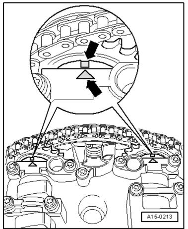
The distance between the two arrows (and thus between the coloured markings) is 15 rollers on the chain.
