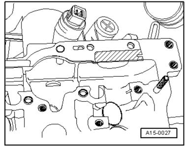
Adjust the colour markings -arrows- so they are aligned.
