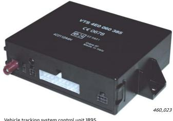
Vehicle tracking system control unit J895
