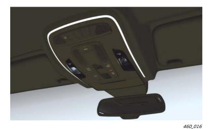
Overhead module with optical fibre
