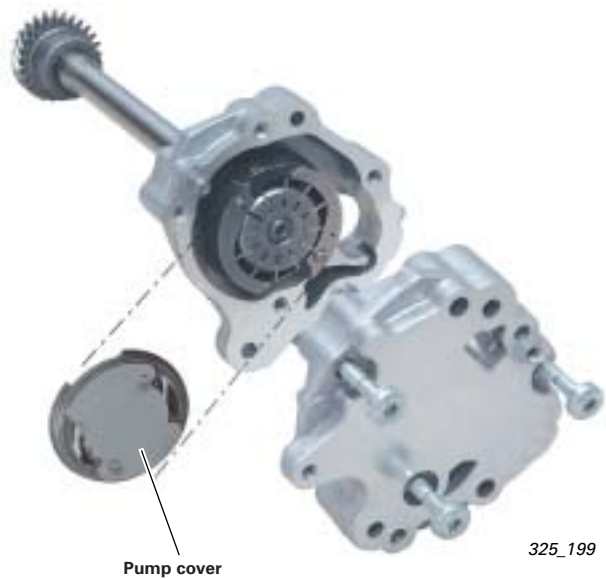
Up-and-down stroke vane-type pump
