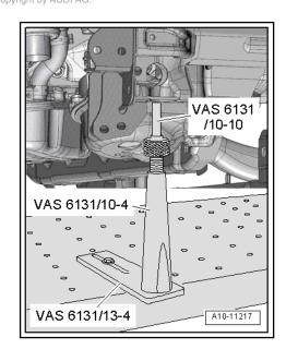
Position support elements from -VAS 6131/10- and -VAS 6131/13- at right of subframe as shown.
