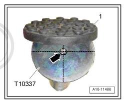
Remove rubber overlay -1- from gearbox support - T10337- .
