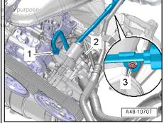
Remove bolts -arrows- and detach power steering pump -1-.
