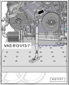
Position the support elements from -VAS 6131/10- and -VAS 6131/12- at left of gearbox, as shown in the illustration.
