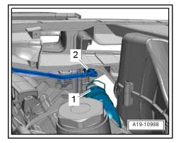
Unplug electrical connector -1- and move wiring harness clear at coolant pipe (front right).
