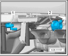
Exhaust flap control unit - J883- / exhaust flap control unit 2 - J945- for vehicles from model year 2014 onwards
