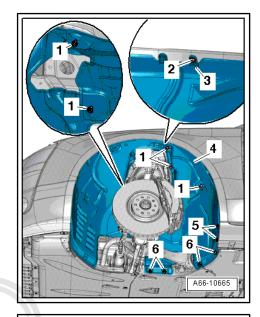
Remove noise insulation panels -1- and -2- ⇒ General body repairs, exterior; Rep. gr. 66; Noise insulation; Removing and installing noise insulation.
