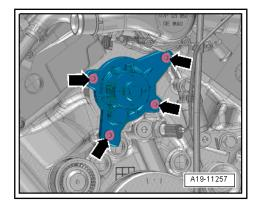
Release fasteners -arrows-, detach release cable -1- from lock carrier and press down.
