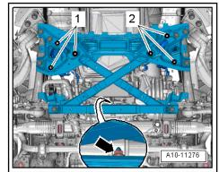
Move clear electrical connectors -1 and 2- for gearbox mounting valves -N262- / -N263-.
