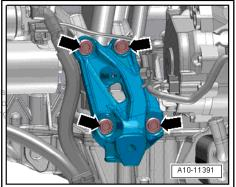
Secure engine with bracket for W12 FSI engine -VAS 6095/1-12- to engine and gearbox support - VAS 6095as shown in illustration and tighten to 40 Nm.
