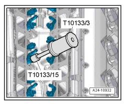
Carefully remove old combustion chamber ring seal -arrow-. To do so, cut open combustion chamber ring seal using knife or prise open with small screwdriver and then pull off forwards.
