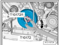
• Marking -2- on vibration damper must align with housing joint -1-.
