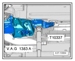
Raise gearbox slightly using engine and gearbox jack - V.A.G 1383 A- .
