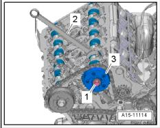
To release chain tensioner, turn tensioning lever in direction of -arrow- and pull off locking pin -T03006-.
