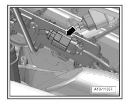
Lift retaining clip -arrow- and disconnect coolant hose (rear right) from engine.
