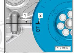
It should then be possible to insert camshaft bar - T10068 Ain slots in both camshafts (both cylinder heads).
