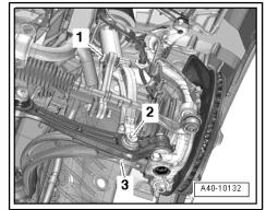
Remove bolts (left and right) -3- securing gearbox mounting strut.
