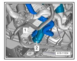
Release hose clip -arrow-, disconnect coolant hose from engine oil cooler and drain off coolant.
