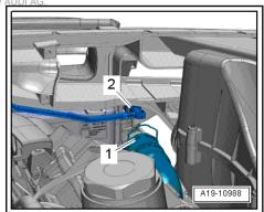
Detach hose -4- for headlight washer system (remove clip -3-).
