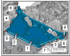
Slacken and remove bolts in the sequence: -22 ... 1-.
