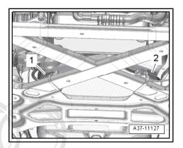
Detach intermediate steering shaft from steering rack and move clear by telescoping upwards ⇒ Running gear, axles, steering; Rep. gr. 48; Steering column; Removing and installing intermediate steering shaft.
