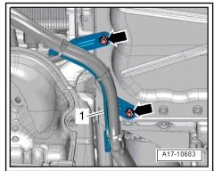
Unplug electrical connector -1- at oil level and oil temperature sender - G266-.
