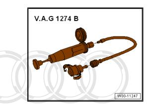
Adapter for cooling system tester - V.A.G 1274/8-
