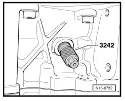
Turn crankshaft two rotations in direction of engine rotation -arrow-.
