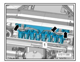
Press release tabs and disconnect relevant secondary air hose -2-.
