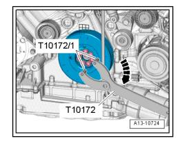
Remove 6 bolts -arrow- for torque converter, turning crankshaft 60° in normal direction of rotation each time.
