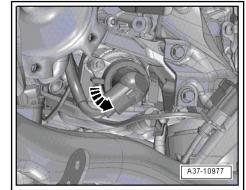
Release hose clip -arrow- and detach coolant hose from coolant pipe (bottom left).
