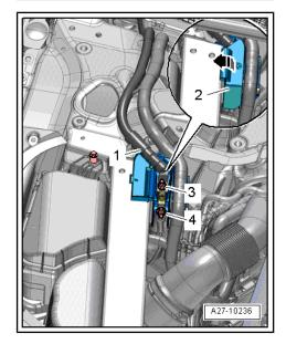
Release retaining tabs -1, 3- and swivel positive terminal -2out of mounting.
