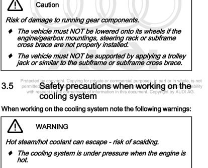
To allow pressure to dissipate, cover filler cap on coolant expansion tank with cloth and open carefully.
