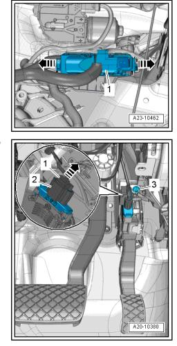
Fitting location of brake light switch - F-
