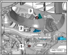
Remove bolts -arrows- from gearbox mounting (left-side) and detach heat shield -1-.
