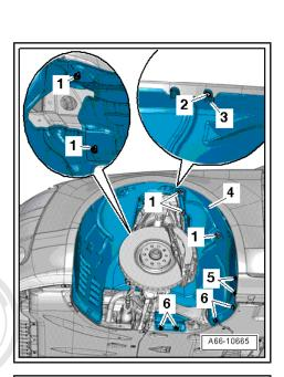
Remove noise insulation panels -1- and -2- ⇒ General body repairs, exterior; Rep. gr. 66; Noise insulation; Removing and installing noise insulation.
