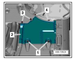
Remove noise insulation panels -1- and -2- ⇒ General body repairs, exterior; Rep. gr. 66; Noise insulation; Removing and installing noise insulation.
