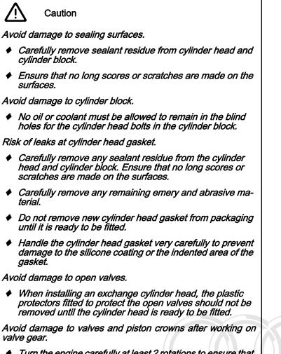
Turn the engine carefully at least 2 rotations to ensure that none of the valves make contact when the starter is operated.
