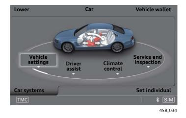
A correctly hitched trailer is detected automatically. In this case, the vehicle is shown in the MMI after pressing the "Car" function key in the "Audi drive select" with towing hitch.
