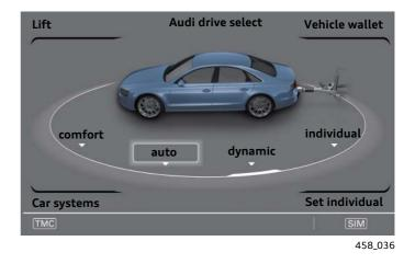
If the trailer is not recognised automatically, trailer operation can be activated by pressing the function keys "Car" – "Car Systems" – "Vehicle Settings" – "Air spring: Trailer" – "On".
