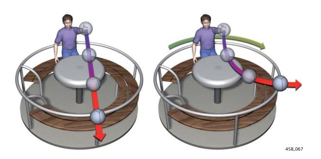
Simplified, the sensor consists of a micromechanical body which is permanently subjected to oscillation excitation. When the vehicle turns, the direction of movement of the oscillating body changes.
