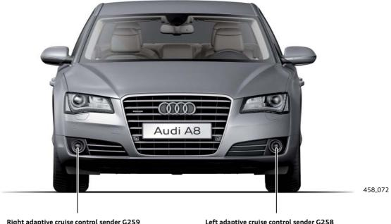
Right adaptive cruise control sender G259 and adaptive cruise control unit J428
