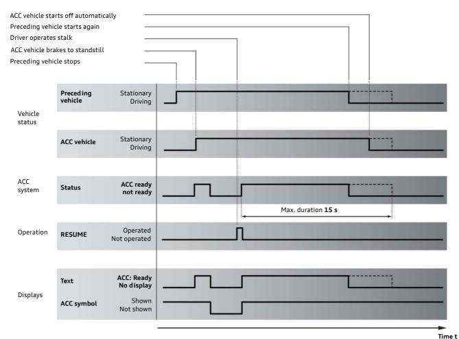
Example of the sequence of control operations in stop & go mode.
