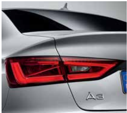
Rear lights, brake lights and rear indicator all featuring LED technology
