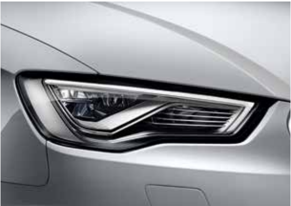
LED headlight (part of LED light package)
