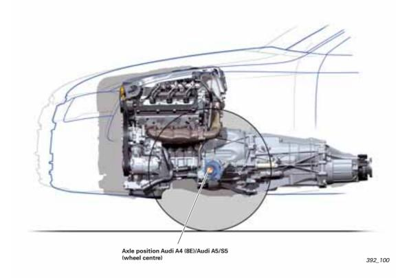
This diagram shows how the specified development goals have been met by virtue of the new engine-gearbox configuration.
