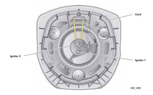
As long as the cord is held in place by the igniter, this discharge port is sealed.
