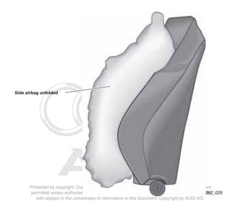
The airbag control unit J234 energises the corresponding side airbag igniter. The ignition charge fired by the igniter in turn ignites the actual propellant charge. The developing gas is cleaned by the metal filter and cooled down, unfolding and inflating the airbag.
