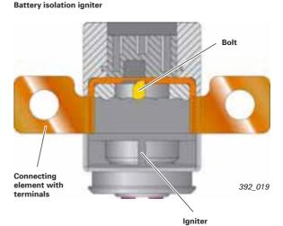
The battery isolation igniter N253 is located in the main fuse box directly on the battery in the boot of the Audi A5.
