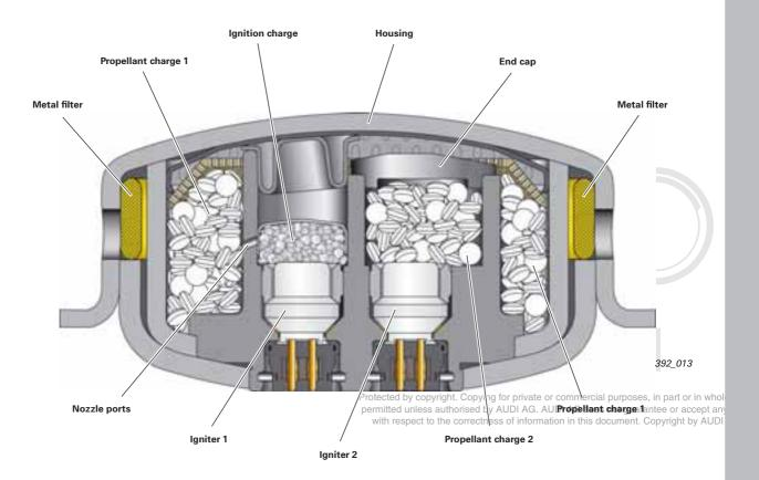
Igniter 1 activated by the airbag control unit J234 fires ignition charge. The actual propellant charge 1 is ignited via nozzle bores.
