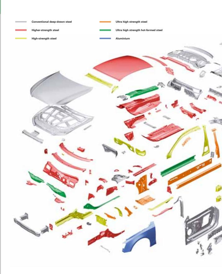
The body construction is a testimony to Audi's experience in lightweight design and its knowledge of innovative welding and joining techniques. Here are examples:
