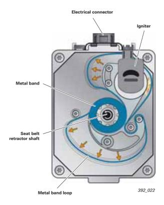
To reduce the pressure losses, the housing cover surface between which the metal band moves is coated with a film of silicone.
