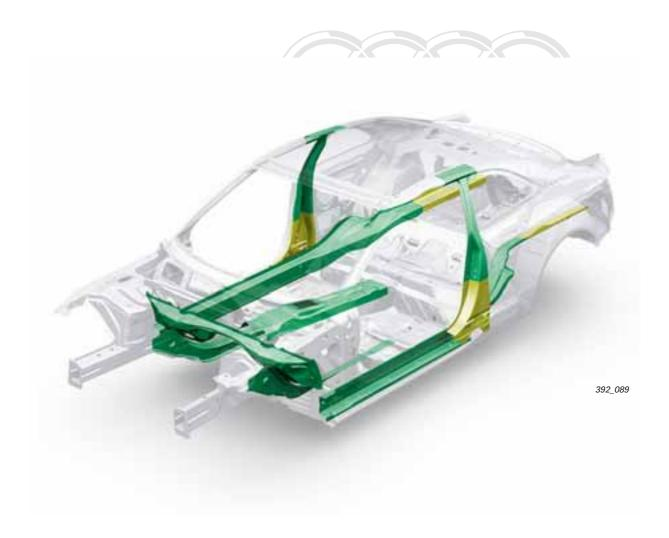
New repair methods are required for the repair of hot formed steel. Straightening and reshaping even of minor deformations are not possible due to the high tensile yield strength and the rebound effect of hot formed steel.
