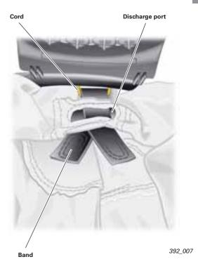
The airbag control unit J234 activates igniter 2. The igniter housing ruptures and the cord is released. The volume of the airbag increases by approx. 4 litres and the additional discharge port is opened. Now more gas can escape through this discharge port when the occupant sinks into the airbag. The airbag is "softer" for the occupants.
