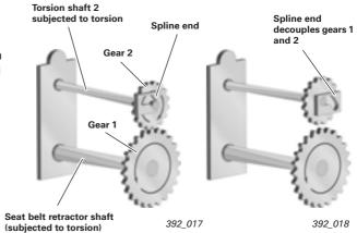
Depending on accident severity and seating position, the airbag control unit J234 decides when the belt force limiter igniter is activated.
