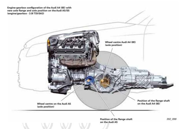
The new engine-gearbox configuration is only possible by moving the front axle drive (differential) forward of the clutch or torque converter.
