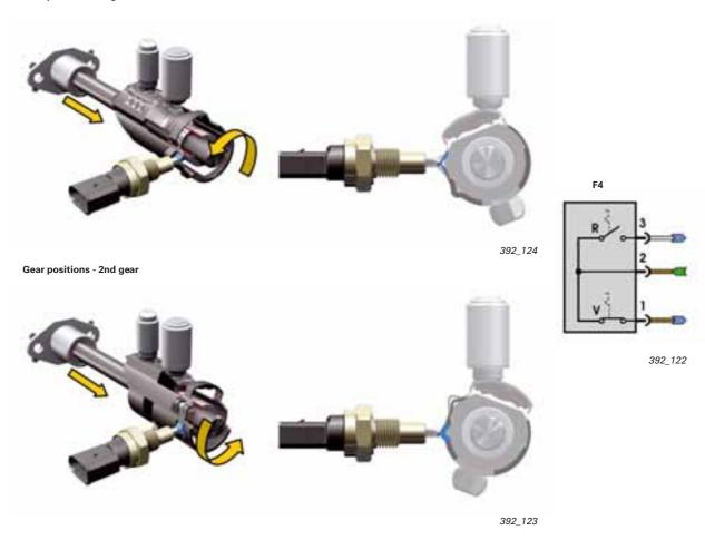
Switch "V" is closed when 1st gear or 2nd gear is engaged (and when reverse gear is engaged). It supplies an earth signal to the onboard power supply control unit J519 (containing the information "1st or 2nd gear engaged/forward drive"). In all other gears, the switch is "open".
