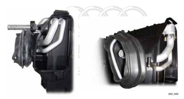
Standard pipe assembly, using the evaporator as an example
