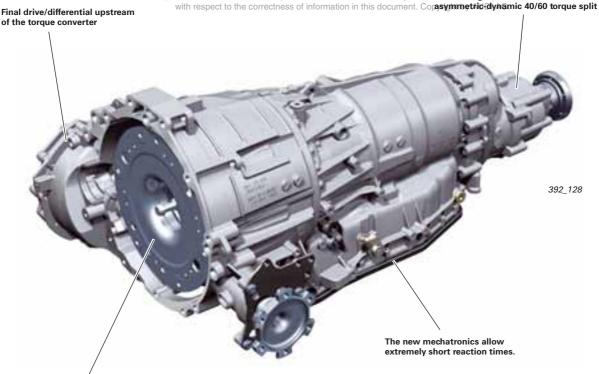
The use of a new two-damper converter in the diesel engine allows the lockup clutch to close earlier. This in turn improves fuel economy and provides a more direct driving dynamic.
