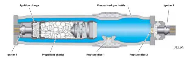
The ignition charge fired by igniter 1 ignites the actual propellant charge. The pressure inside the pressurised gas bottle increases, bursting rupture disc 1 at a certain pressure. The gas mixture inflates and unfolds the airbag.
