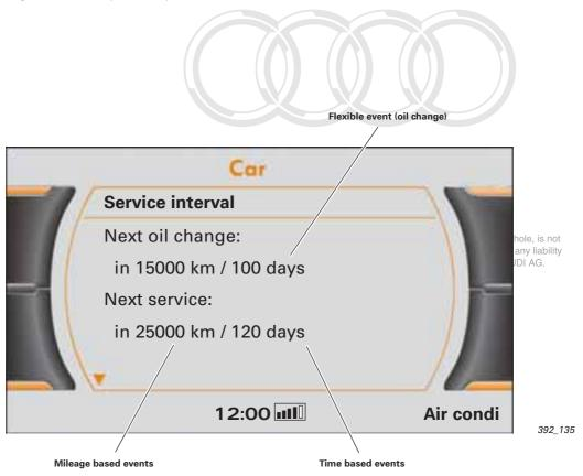
Since time and mileage based service events are now indicated, process reliability is higher. This means that there is no danger of service events being missed without the customer receiving prior warning. The requirement for this is that the Service Interval Display is reset correctly.
