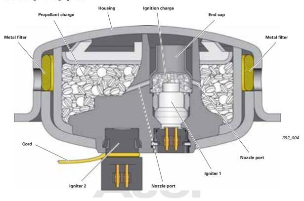
An additional igniter, driver side airbag igniter of N250.cis attached to the back of the lairbag. A cord which seals an additional discharge poet is wrapped around this igniter of guarantee or accept any liability with respect to the correctness of information in this document. Copyright by AUDI AG.
