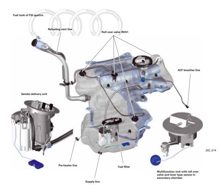
If servicing is required, two fuel delivery units are available as spare parts. A distinction is made here between petrol and diesel engines. The quattro variant is always supplied in combination with a pre-heater. In this case, the unused terminals are sealed using cell plugs and dummy plugs. These plugs can be ordered from the electronic parts catalogue (ETKA). The fluid level sensors, the suction jet pumps and the fuel filter are also available as replacement parts.
