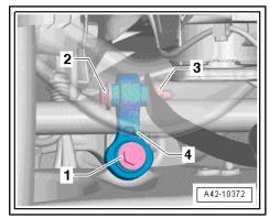
Check anti-roll bar bush -1- for damage.
