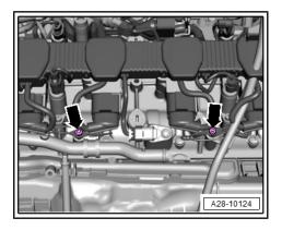
Loosen hose clips -arrows- and detach air pipe.
