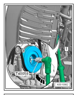
Turn poly V-belt clockwise using reversible ratchet and adapter - T40058- , and check pulley for air conditioner compressor -3- and entire belt. Look for the following types of damage:
