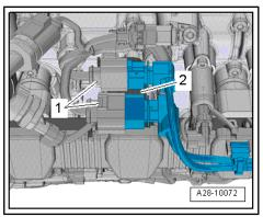
Unplug electrical connectors -arrows- and move wiring clear.
