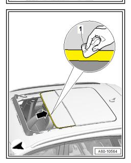
Use a paintbrush to lubricate inside of guide rail -arrow- with lubricating paste - G 060 751 A2- .
