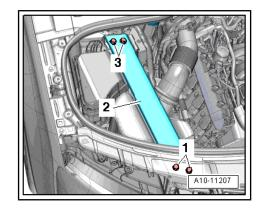
Remove securing bolts -arrows- and detach air cleaner (top section).
