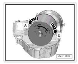
Check for dirt in housing and water drains -arrow- and clean if necessary <u>⇒ page 122</u>.
