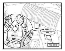
Use extraction hose included in brake filling and bleeding equipment - VAS 5234- to extract brake fluid from reservoir (with strainer installed) until fluid is level with bottom edge of strainer. Make sure that no more fluid flows back into reservoir from strainer after extracting fluid.
