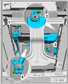
Check by hand that battery -A- and second battery -A1- are securely installed. If necessary tighten securing bolts -2- and -3- on shared retainer plate -1- on battery base to specified torque (see table of tightening torques for installation ⇒ page 31 ).
