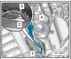
Turn filter element in anti-clockwise direction -arrow A- and remove it.
