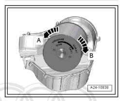
Check for dirt in housing and water drains -arrow- and clean if necessary <u>⇒ page 122</u>.
