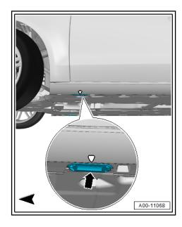
Rear: Position support plates of lifting platform under plastic mountings -arrow- on underside of side member trim.
