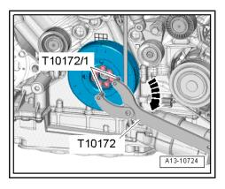
Turn poly V-belt clockwise using counterhold tool - T10172and check pulley for air conditioner compressor -7- and entire belt. Look for the following types of damage:
