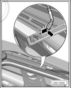
Use a paintbrush to lubricate outside of guide rail -arrow- with lubricating paste - G 060 751 A2- .
