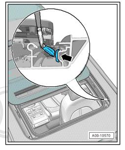
Remove grease and dirt from front and side edges of glass panel -arrows- using cleaning solution - D 009 401 04- and a lint-free cloth.
