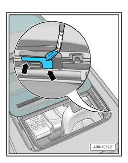
Use a paintbrush to lubricate top guide rail of glass panel -arrow- with lubricating paste - G 060 751 A2- .
