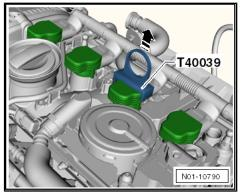
Unscrew spark plugs from cylinder head using spark plug socket - VAS 3122B- .
