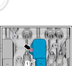
Insert puller - T10530- into hole -1- of ignition coil and turn knurled nut -2- clockwise until puller is secured in place.
