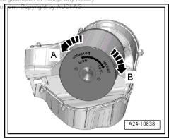
Check for dirt in housing and water drains -arrow- and clean if necessary ⇒ page 122.
