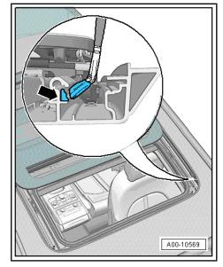
Use a paintbrush to lubricate bottom guide rail of glass panel -arrow- with lubricating paste - G 060 751 A2- .
