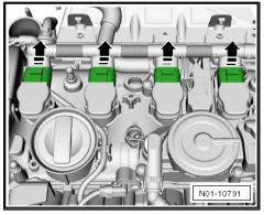
Position puller - T40039- on thick rib at top of ignition coils and detach all ignition coils from spark plugs one after the other in direction of -arrow-.
