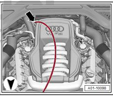
Attach both charger clamps to wire (see -illustration-) and guide upwards into engine compartment.
