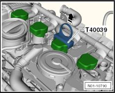
Unscrew spark plugs using spark plug socket and extension -VAS 3122B-.
