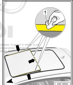
Use a fine-pored sponge -1- to lubricate glass panel seal at front -arrow- with Krytox lubricating paste - G 052 141 A2-Make sure that no coarse residue remains visible after applying lubricant.
