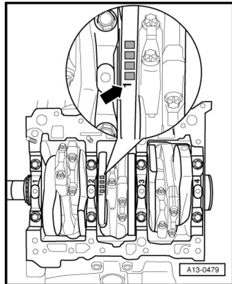
**Installing crankshaft bearing caps**
