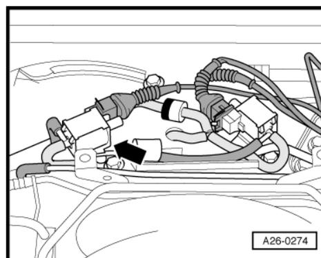
**Fitting location of secondary air pump motor -V101-**
