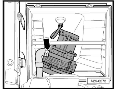
**Fitting location of secondary air pump relay -J299-**
