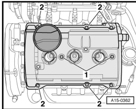
**1.4 Removing and installing right cylinder head cover**
