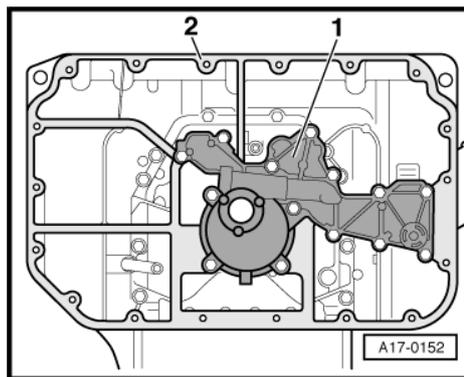
**1.6 Installing bottom part of sump - engines with liquid gasket**
