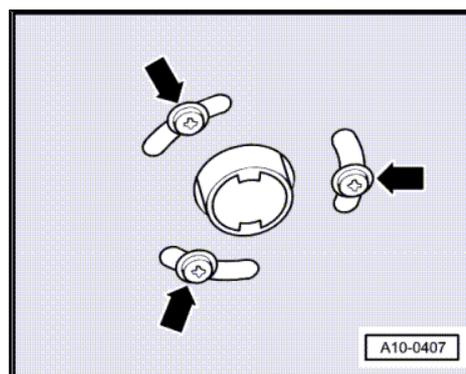
– Release fasteners -1- and detach noise insulation.
