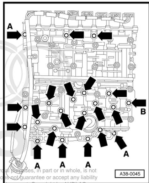
**Internal wiring harness in gearbox with integrated gearbox oil (ATF) temperature sender -G93-**
