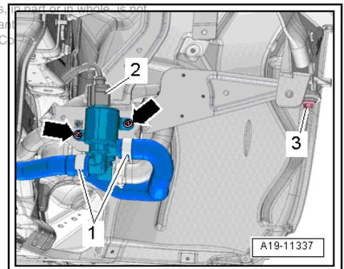
**Fitting location of gearbox oil cooling valve -N509-**
