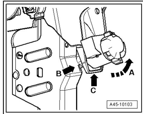
**Fitting location of radiator outlet coolant temperature sender -G83-**
