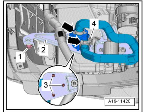
**Fitting location of charge air cooling pump -V188-**
