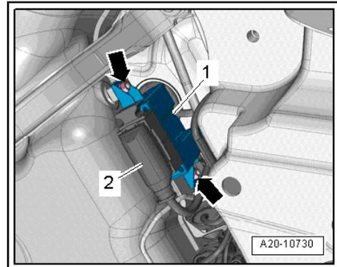
**Fitting location of secondary air pump motor -V101-**
