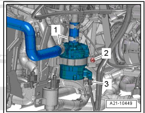
**Fitting location of coolant valve for gearbox -N488-**
