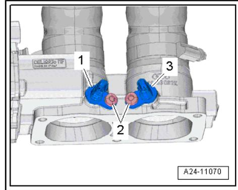
**Fitting location of fuel pump control unit -J538- -1-**
