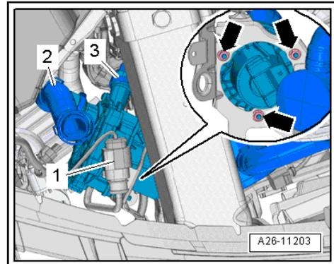
**Fitting location of sender 1 for secondary air pressure -G609-**
