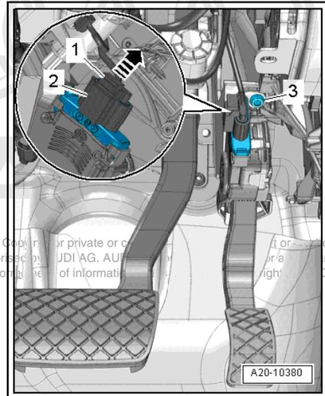
**Fitting location of brake light switch -F-**
