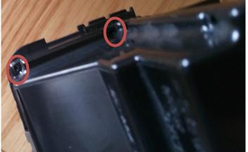
The front panel can now be taken from the case by lifting the four tabs, two on the top and two on the bottom.
