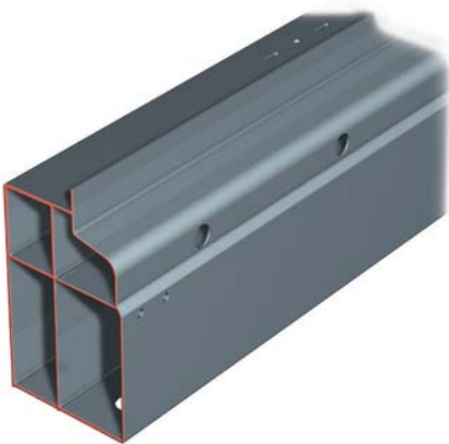
Sill section, Audi TT Four-chamber extruded section
