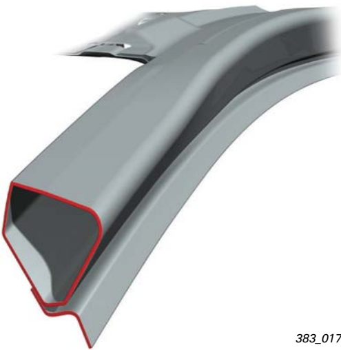
A-post, Audi A8 Single-chamber extruded section
