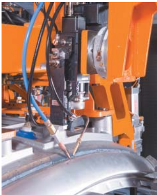
Laser welding process in production
