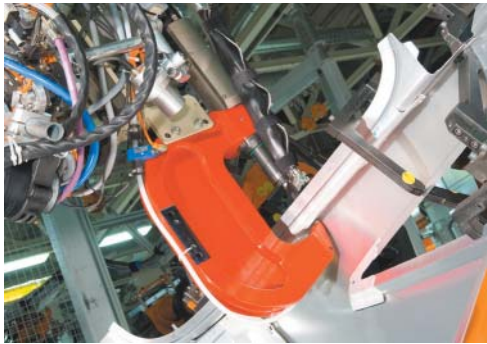
Solid punch riveting process in production
