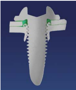
Micrograph of a Flow Drill screw connection
