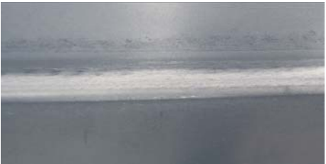
Laser weld seam before (above) and after the brushing process (below)
