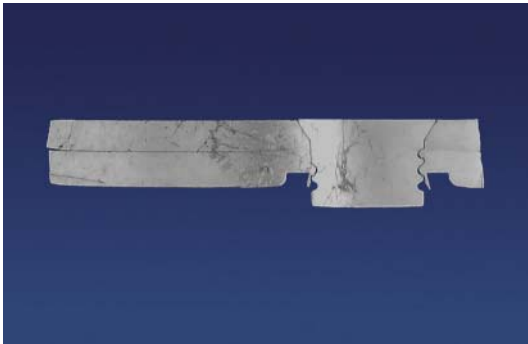
Micrograph of a solid punch riveted joint
