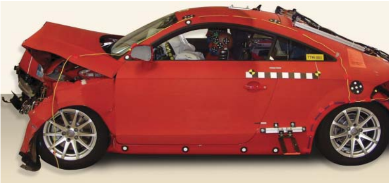
Euro NCAP head-on collision (64 kph with partial overlap)
