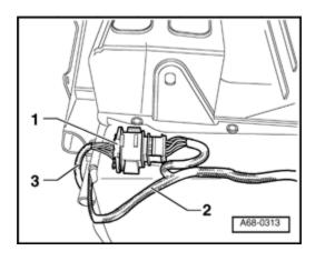
Disconnect electrical harness connector - 1 - for glove compartment wiring harness - 2 - from lead wire - 3 - .
