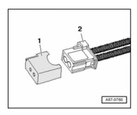
Seal the open wiring set connector - 2 - for fiber-optic cable using Protective Cap For Cable Connector VAS 6223/9 - item 1 - .
