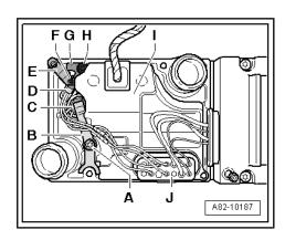
Measure resistance between contact "10" and contact "11" at black wires.
