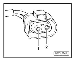
Assignment of contacts in 2-pin connector (in-vehicle wiring to auxiliary heater control unit - J364-)
