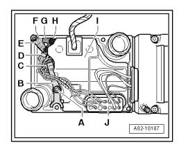
Measure resistance between contact "7" and contact "8" at white wires.
