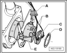
Press wires of combustion air blower - V6- in contacts 13 and 14 out of 14-pin connector housing.
