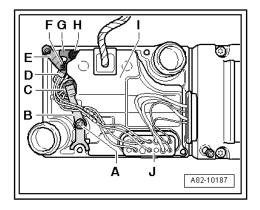
Press wires of glow plug for heater - Q9- in contacts 3 and 6 out of 14-pin connector housing.
