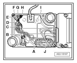
Press wires of flame monitor - G64- in contacts 1 and 2 out of 14-pin connector housing.
