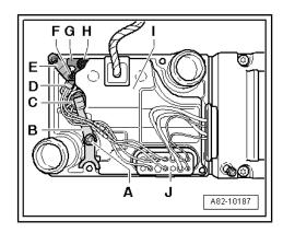
Press wires of temperature sensor 2 for supplementary and auxiliary heating - G587- in contacts 7 and 8 out of 14-pin connector housing.
