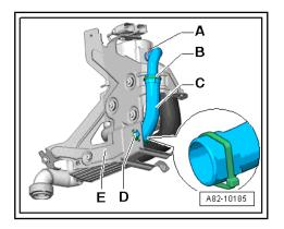
Secure intake air noise insulation -C- at locations provided on bracket -E- with cable ties -B- and -D-.
