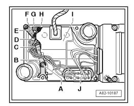
Measure resistance at connector between contact "13" and heater housing.
