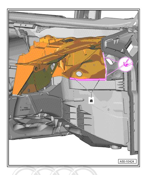
Remove remaining material from node casting using compact angle grinder .
