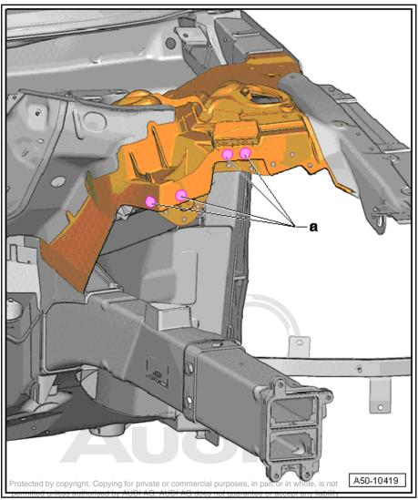
Match up support for inner suspension strut mounting at points -a- and mark holes using plastic hammer. Then match up at points -b- and mark holes using plastic hammer.
