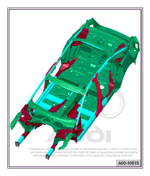
The outer side panel and roof are removed to give a clearer illustration. These panels are made of sheet aluminium.
