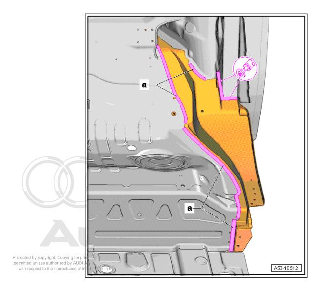
Release inaccessible rivets -a- using dent remover for aluminium vehicles - VAS 5196- .
