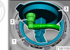
Remove locking ring using wrench - T10202- . \_
