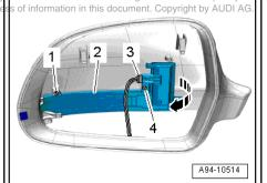
Release retainers -arrows A- and press lane change assist warning lamp -1- out of exterior mirror housing -2- -arrow B-.
