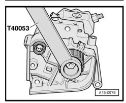
Pull toothed belt sprocket off high-pressure pump using puller -T40064-.
