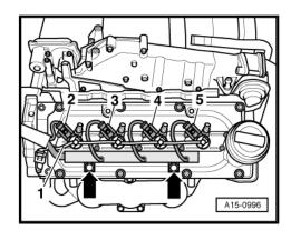
Remove nuts securing injectors on both cylinder heads -arrows-.
