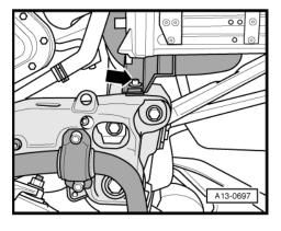
Remove bolts -arrows- and detach bracket for charge air cooler (right-side).
