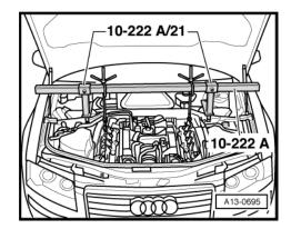
... until cylinder head cover is just slightly above bracket for torque reaction support -arrow-.
