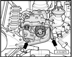
Remove central nut for high-pressure pump (use counterhold tool - T40053-).
