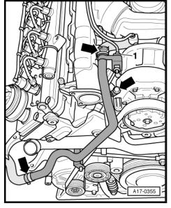
Unbolt exhaust gas recirculation valve - N18- -1- and exhaust gas recirculation valve 2 - N213- -2- from intake manifolds.
