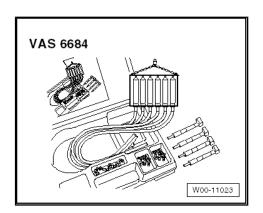
♦ Lengths of hose to fit return line connections on injectors
