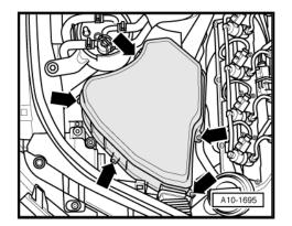
Cover air mass meter -1- with a clean cloth and clean out bottom and top sections of air cleaner housing.
