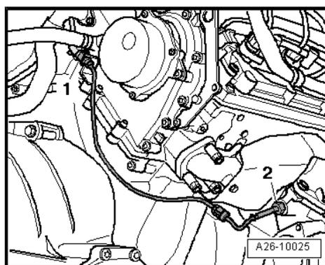
**Exhaust gas temperature sender 1, bank 2 - G236- in turbocharger (left-side) (cylinder bank 2)**
