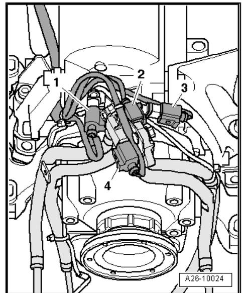
**Temperature sender 2 before particulate filter - G498- -2-**
