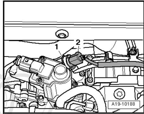
**Charge pressure sender - G31- with intake air temperature sender - G42-**
