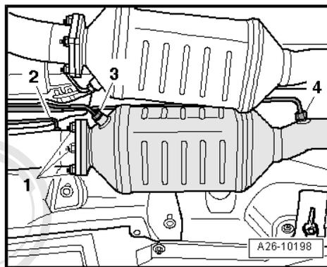
**Lambda probe 2 - G108- and exhaust gas temperature sender 2, bank 2 - G449-**
