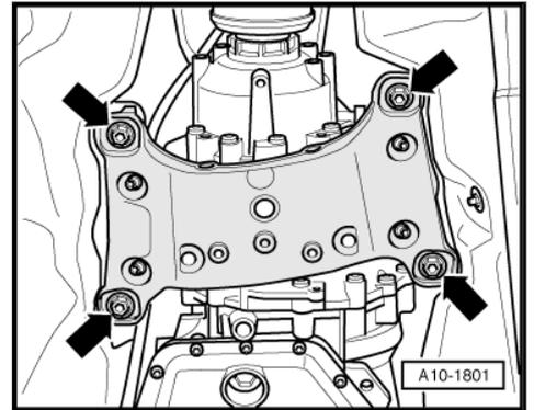
Adjust mounting for torque reaction support before tightening torque reaction support:
