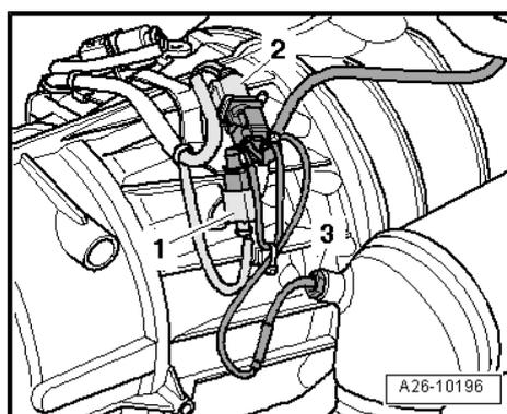
**Exhaust gas temperature sender 1 - G235- in turbocharger (right-side) (cylinder bank 1)**
