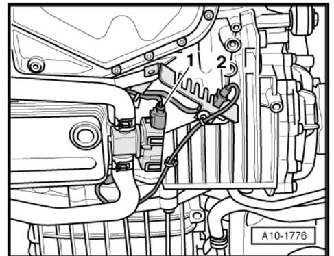
**Oil temperature sender - G8- and oil pressure switch - F1-**
