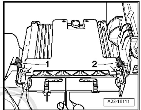
The threads of the two shear bolts -4- which are not screwed into the engine control unit are secured with locking fluid. To unscrew these two bolts, the threads must therefore be heated with the hot air blower.
