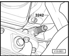
Remove vibration damper on injection pump sprocket (bolts -1-).
