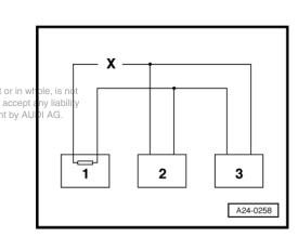
The faults entered in the fault memories indicate that there is no connection between control unit 2 and control units 1 and 3.
