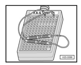
Connect hand-held multimeter to measure voltage on connector for injection pump to following contacts of wiring harness. (Test leads remain connected).
