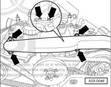
Turn engine until the marking "- OT -" (TDC) is visible on cam-
