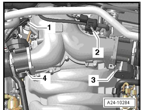
**Variable intake manifold changeover valve -N335- -1-**
