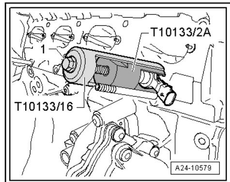
**Renewing combustion chamber ring seal (teflon ring seal)**
