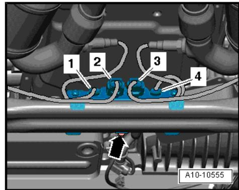
**Fitting location of electrical connectors for Lambda probes -G286- and -G108-**
