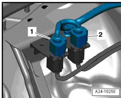
– Unscrew relevant Lambda probe using tool from Lambda probe open ring spanner set -3337- .
