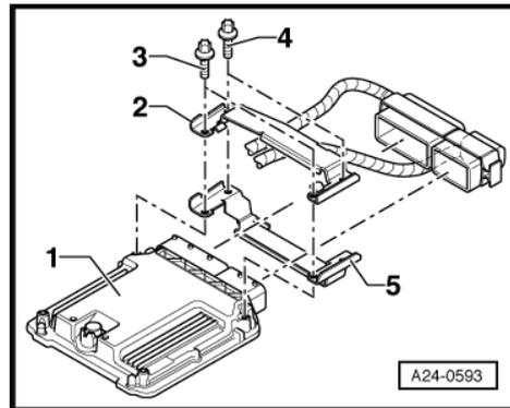
The threads of the two shear bolts -3- which are screwed into the engine control unit are not secured with locking fluid. Do not apply heat to the threads in the control unit housing; this is not necessary and would cause overheating of the control unit.
