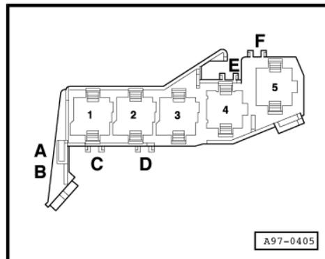
**Relay and fuse holder behind dash panel (left-side)**
