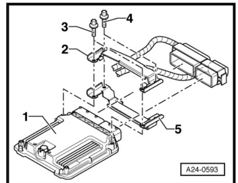
The threads of the two shear bolts -3- which are screwed into the engine control unit are not secured with locking fluid. Do not apply heat to the threads in the control unit housing; this is not necessary and would cause overheating of the control unit.
