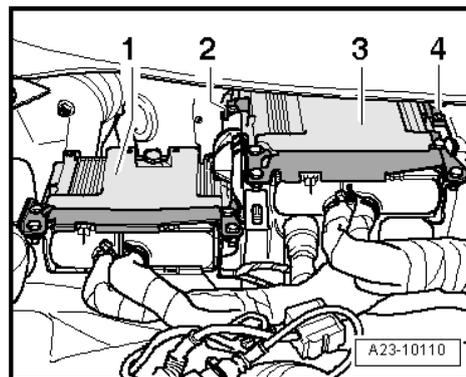
**5-position relay carrier in passenger's footwell**
