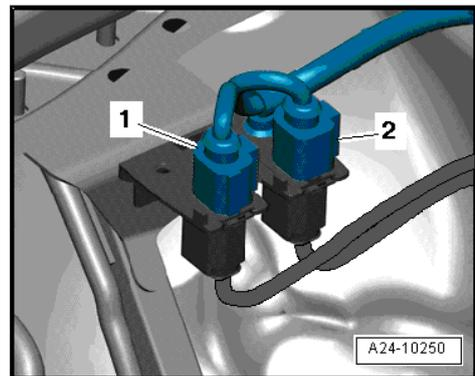
**Fitting location of electrical connectors for Lambda probes -G287- and -G130-**
