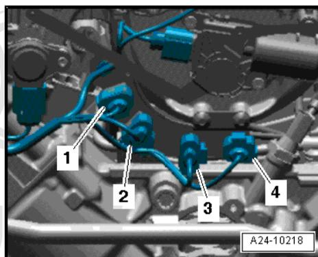
– Unplug electrical connectors for fuel metering valve -N290- and fuel metering valve 2 -N402-.
