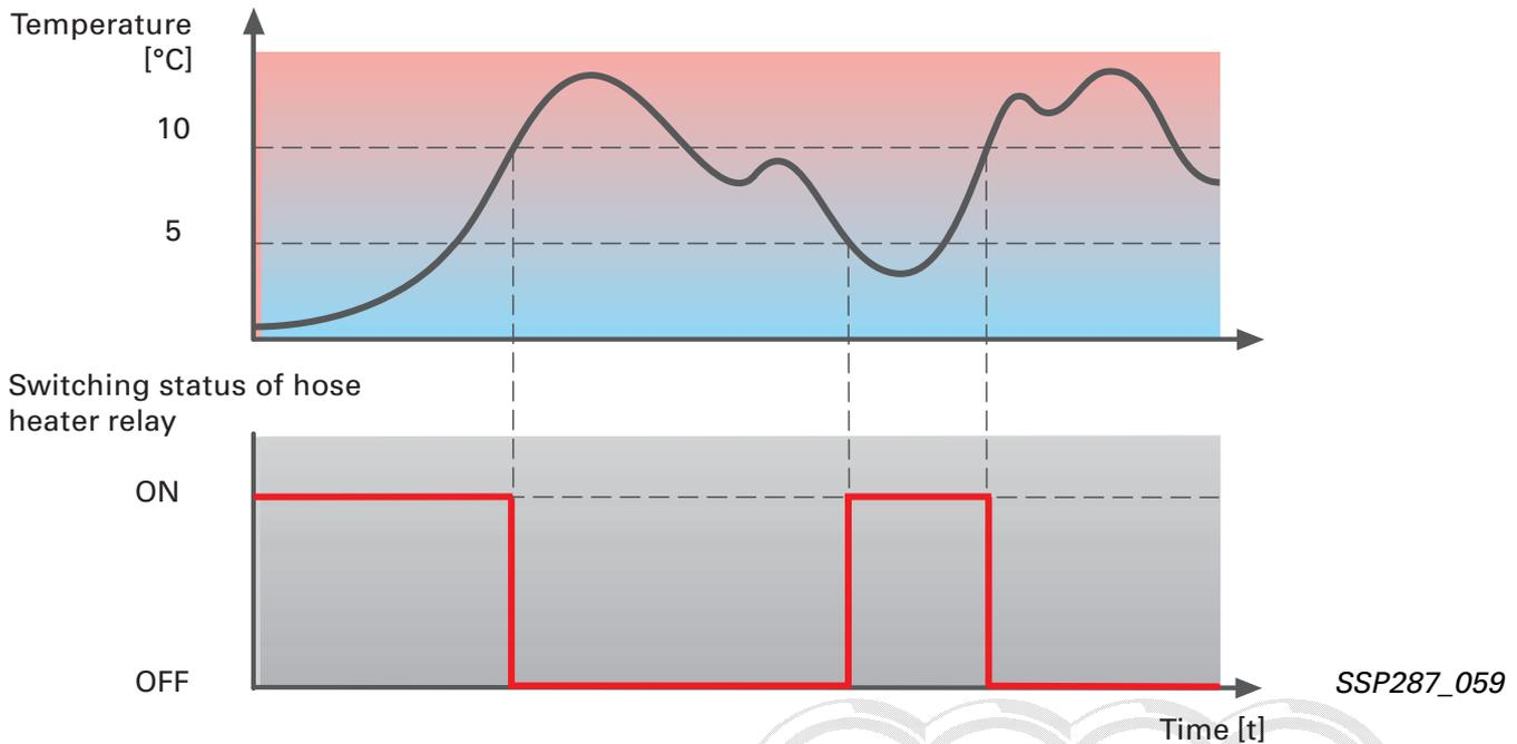
The windscreen washer system hose heater is actuated via a relay energised by the onboard power supply control unit 2 J520.
