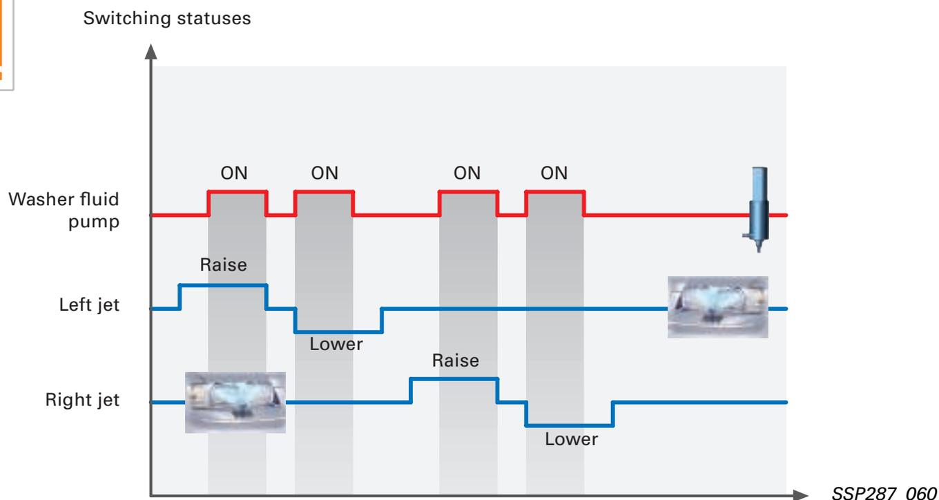
The onboard power supply control unit 2 J520 actuates one washer fluid pump and two pop-up washer jet motors. The washer fluid pump is actuated via the headlight washer system relay J39, which is energised by the onboard power supply control unit 2.
