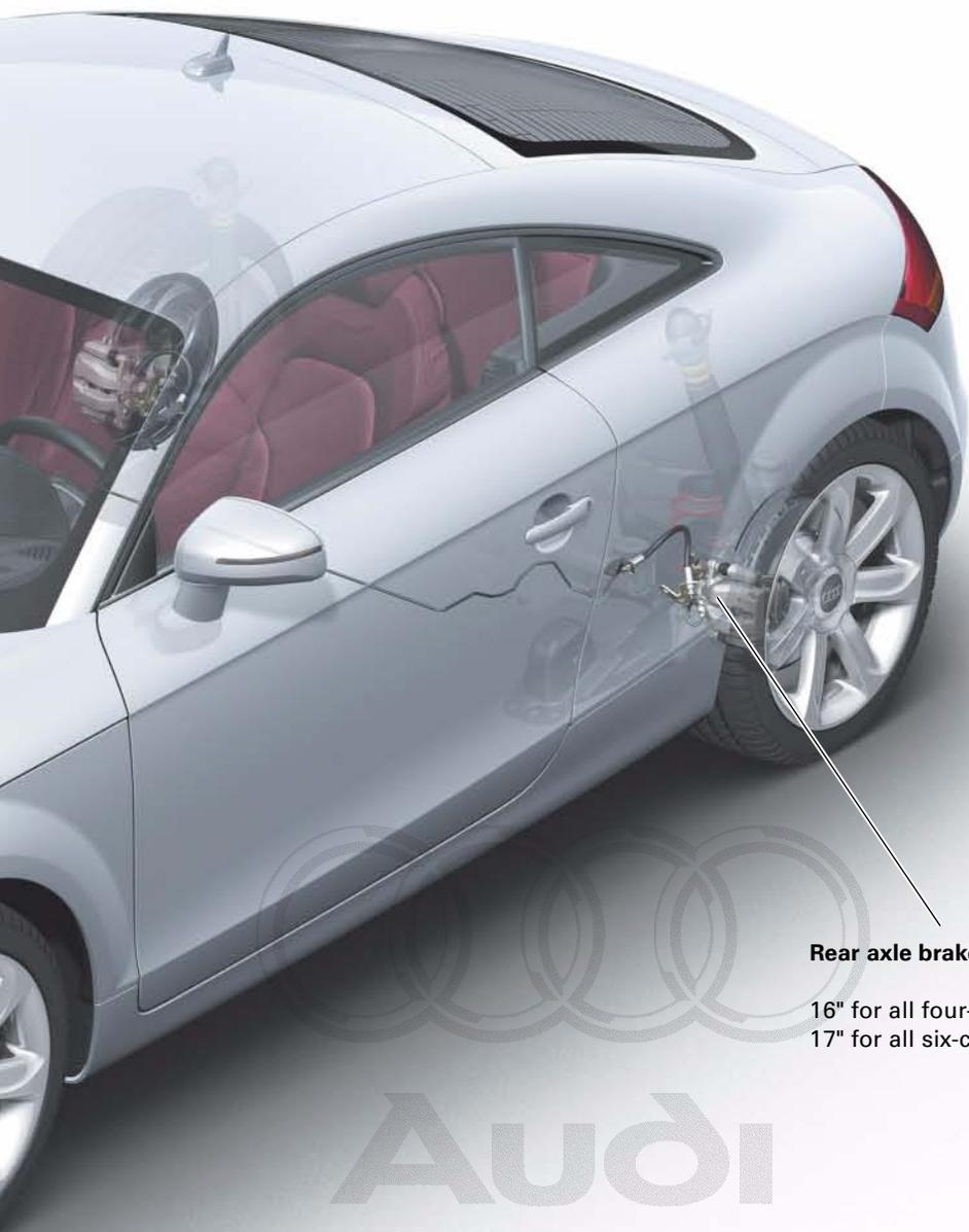
**Rear axle brake caliper**
