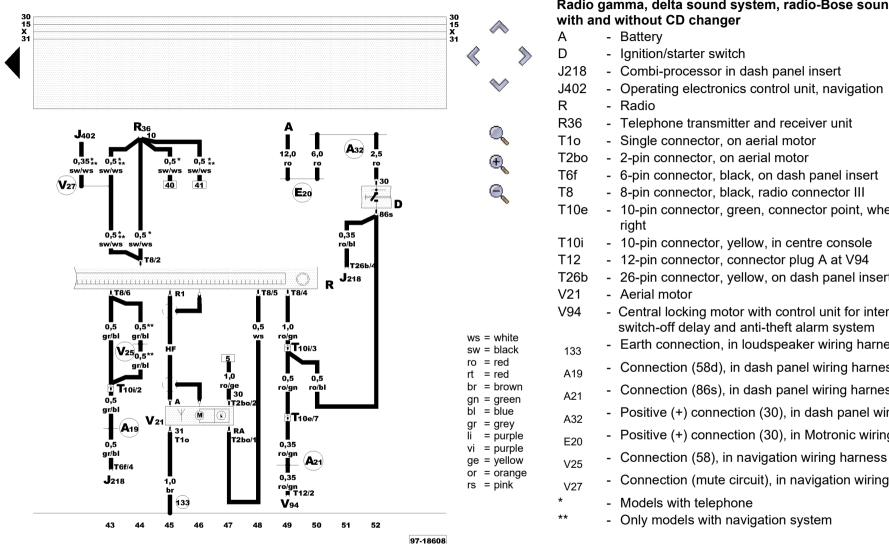
Radio gamma, delta sound system, radio-Bose sound system
