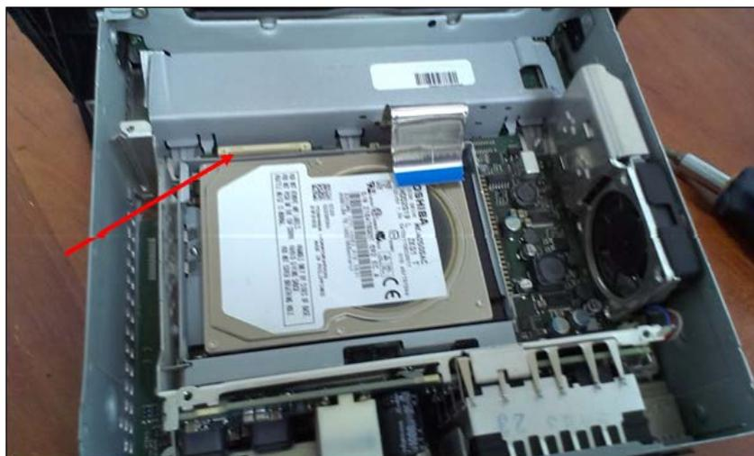
There is a small pin that holds the drive, just gently push in the clip (where the arrow is pointing in the above picture) and the drive should pop out.
