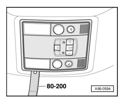
Insert removal lever -80 - 200between housing of interior
