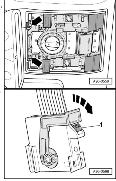
Press retaining tab -1- at multi-pin connector.
