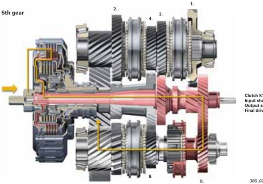
Clutch K1 Input shaft 1 Output shaft 2 Final drive/differential
