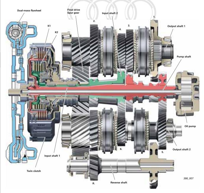
Engine torque is transmitted through a dual-mass flywheel to the twin clutch input hub by means of a stub shaft spline.
