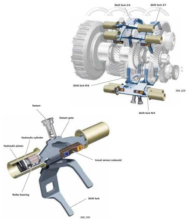
The shift forks are pressurised in such a way that, depending on requirements, they move to the left/ right stop (corresponding gear selected) or to the middle position (neutral position).
