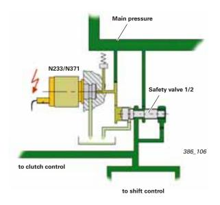
When the electromagnetic pressure control valve N233 (N371) is energised, the control pressure acts on the respective safety valve. The gate is moved to the right against the spring force. In this position it opens the pressure supply to the clutch and shift control systems.
