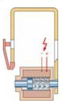
If the selector lever is in position "N" for longer than 2 seconds at "ignition ON", then N110 is energised by the selector lever sensor system E313. The lokking bolt is moved into the neutral "N" pawl against the pressure of the spring. The N lock is not activated when the vehicle is travelling faster than approx. 5 kph.
