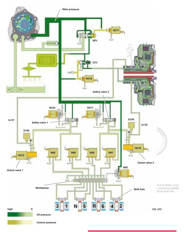
A special feature of the 02E gearbox is the direct activation of clutches K1 and K2 by electromagnetic pressure control valves.
