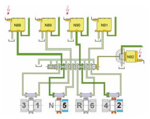
The following shift forks/gears can be activated when N92 is energised:
