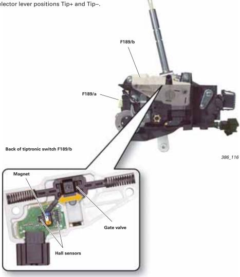
The information from F189/a and F189/b is evaluated by the selector lever sensor system and transmitted to the mechatronic control unit by CAN message.
