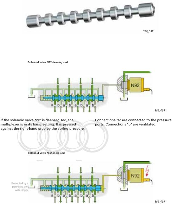
When the solenoid valve N92 is energised, the multiplexer is pressed against the left-hand stop by the control pressure.
