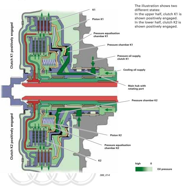
Pressure oil is supplied to the clutches through the main hub by means of rotating ports. Rectangular rings provide a tight seal between the housing and the main hub. The oil flows along ducts in the main hub to the respective points. Protected by copyright copyright for provide or commercial purposes, in part or in whole, is sholl.
