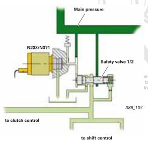
Pressure control valves N233 and N371 have a rising current/pressure characteristic.
