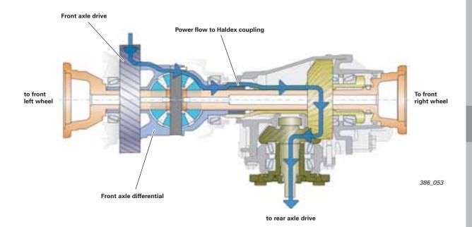
The speed of the front axle drive is increased by a factor of 1.6 in the bevel box and transmitted to the Haldex coupling by prop shaft. The increase in speed improves the response of the Haldex coupling. Torque is reduced, thereby allowing a smaller prop shaft design to be used. Speed is then reduced by a factor of 1.6 in the rear axle drive.
