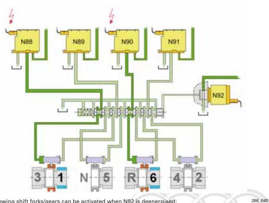
The following shift forks/gears can be activated when N92 is deenergised:
