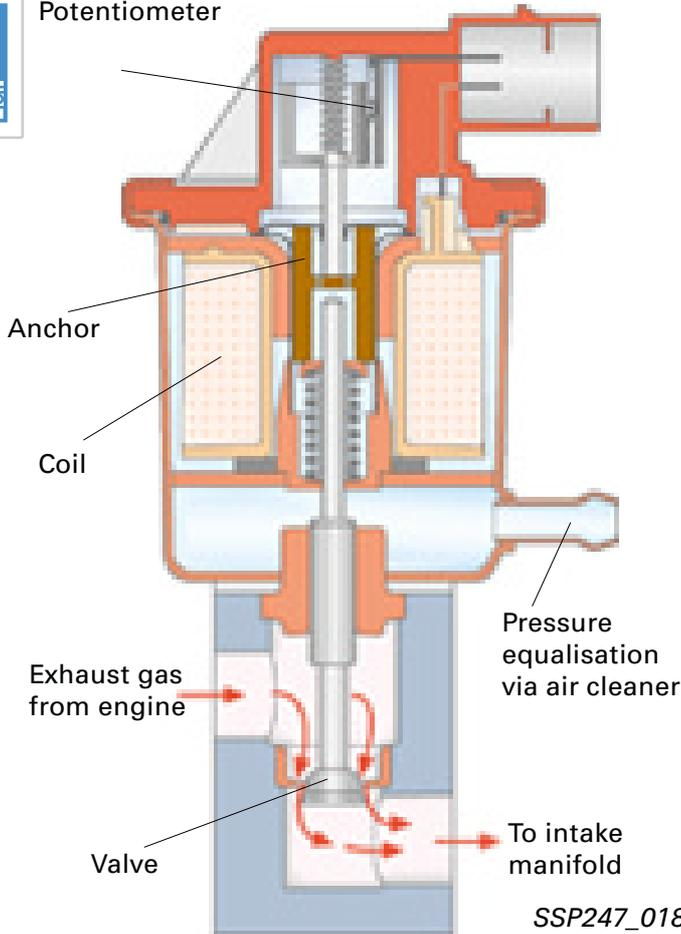
The EGR valve terminates (zero-current process) the recirculation of exhaust gases to the intake manifold. It is switched on from a coolant temperature of 35 °C.
