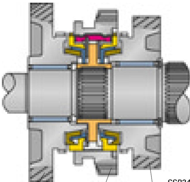
The double synchronisation improves the smoothness of the gear change from 3rd gear down to 2nd and from 2nd gear down to 1st.
