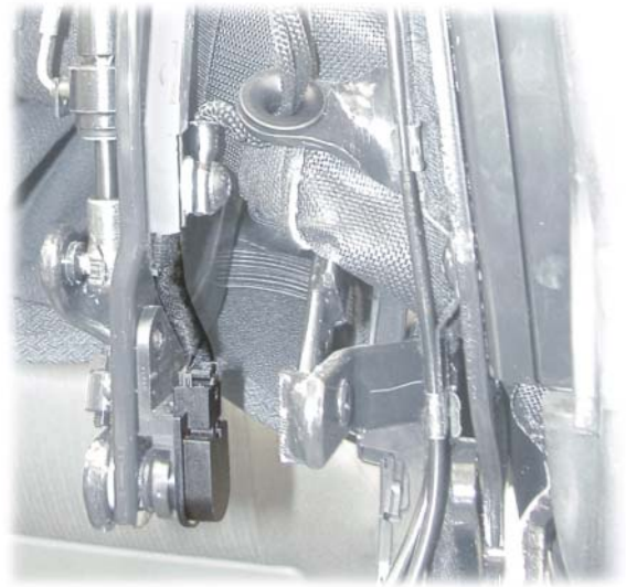
Convertible top frame position sender G356
