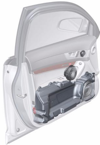
Audi A6 '05 front door with subwoofer and loudspeaker installation positions
