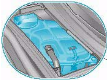
Coolant expansion tank
