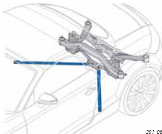
Attachment of the diagonal struts for quattro four-wheel drive
