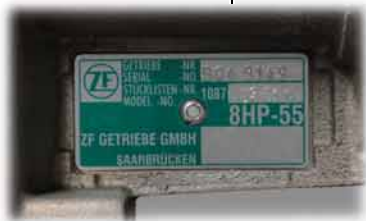
The rating plate is located below the flange shaft (visible from below)
