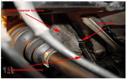
Once it is loose you can turn it with your fingers. Remove the washer under the nut you just removed. The transmission mount stays here for now.
