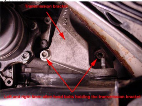
These are simple. Remove the left one with the same 8mm hex head socket (tool C)on your long extension (tool J). Note the left one is longer than the others. The right most hex bolt is right above the transmission mounts threaded shaft.
