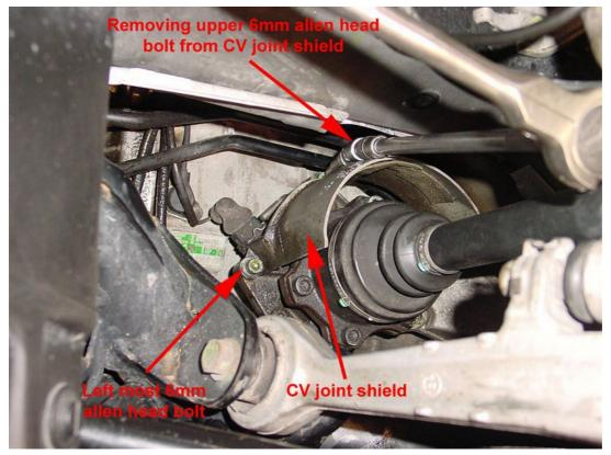
Remove shield. Access to the transmission support bracket will now be easier from the wheel well now.
