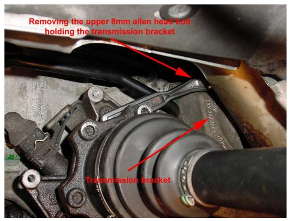
With just the 8mm hex head socket (tool C) in hand, I reached up and placed it into the bolt. Then I stuck my shorter craftsman 3/8 drive ratchet (tool K) on it. The motion to remove it is pretty easy, just pull it down to loosen it. Once it gets loose you can unscrew it with your fingers.
