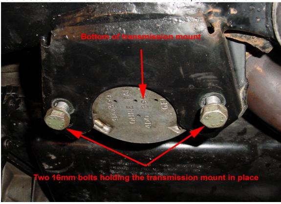
Once both are removed (using either tool A or tool I), and if the transmission bracket is out of the way, you can angle the transmission mount down and out of the car.
