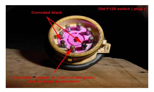
Old F125 switch, notice the corrosion on the contacts.
