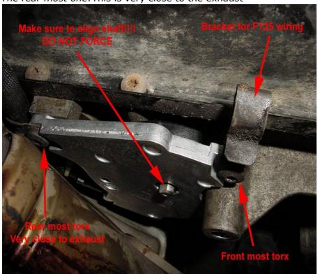
I chose to grind down the correct size torx instead of removing the exhaust header. I spent 2 minutes on the grinder, much easier than taking the exhaust off.
