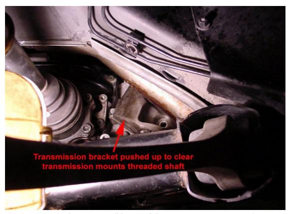
There is a way to place it so it will be out of the way, so you can remove the transmission mount easily during the next step.
