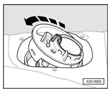
→ Hold flange in fitting position approx. 40 mm over opening.
