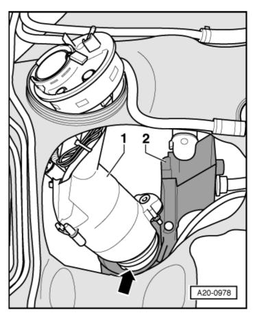
→ Now turn fuel delivery unit anti-clockwise 45°, which will lower the delivery unit into the fuel tank.
