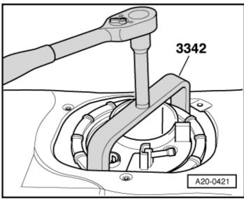
–  $\rightarrow$  Tighten securing bolt -arrow- to 20 Nm.
