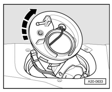
→ Now turn fuel delivery unit anti-clockwise 45° while pulling upwards...
