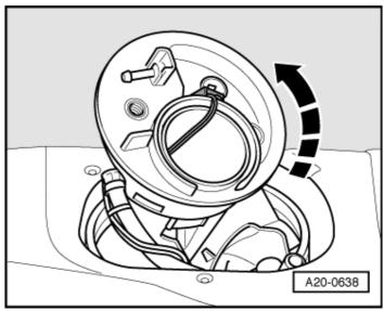
$^- \to \text{Turn}$  the fuel delivery unit anti-clockwise  $45\,^{\circ}$  further to its fitting position.
