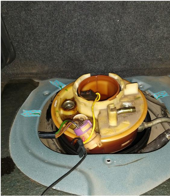
Lift the housing straight up whilst turning gently left and right. This releases the housing from the plate at the bottom of the tank. Then turn the housing anti-clockwise whilst lifting.
