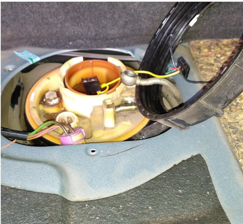
The collar which secures the pump housing to the top of the fuel tank is ready to be removed once the two fuel lines have been disconnected.
