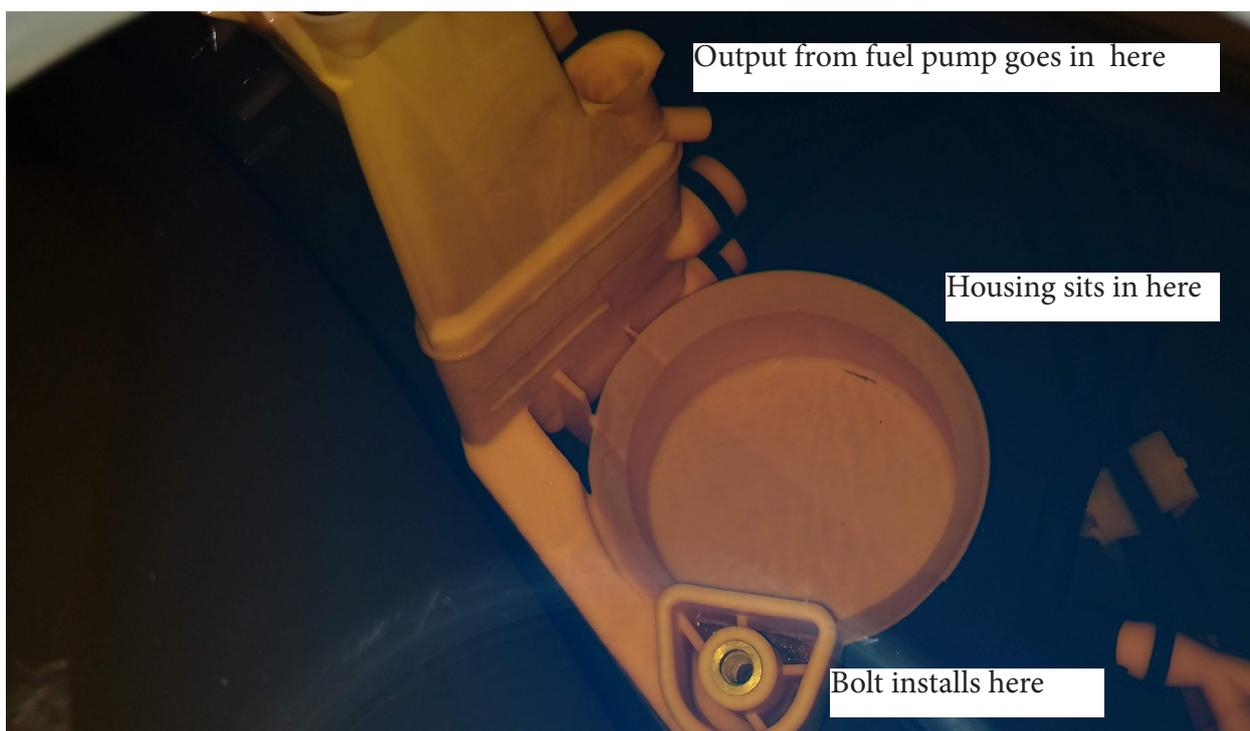
Here is what you must achieve to ensure the housing has been located correctly.
