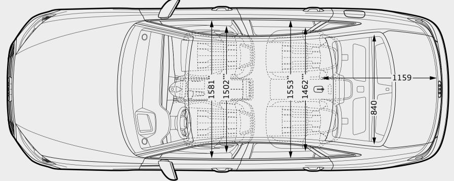
Dimensions in millimetres. Optional equipment may affect dimensions. Dimensions were measured with vehicle at unladen weight. Turning circle approx. 12.5m. \*Maximum headroom. \*\*Elbow room width.\*\*\*Shoulder room width.
