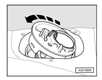
•  $- \rightarrow$  Hold flange in fitting position approx. 40 mm over opening.
