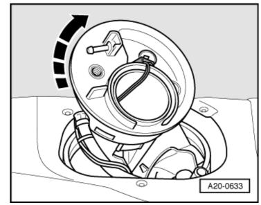
•  $- \rightarrow$  Now turn fuel delivery unit anti-clockwise 45° while pulling upwards...
