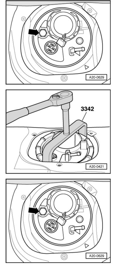
•  $- \rightarrow$  Fit locking ring and tighten to 70 Nm using special tool 3342.
