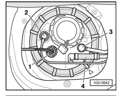
•  $- \rightarrow$  Unscrew and remove union nut with special tool 3342.
