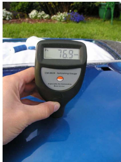
Paint thickness reading on struck through area of Peugeot 307 door
