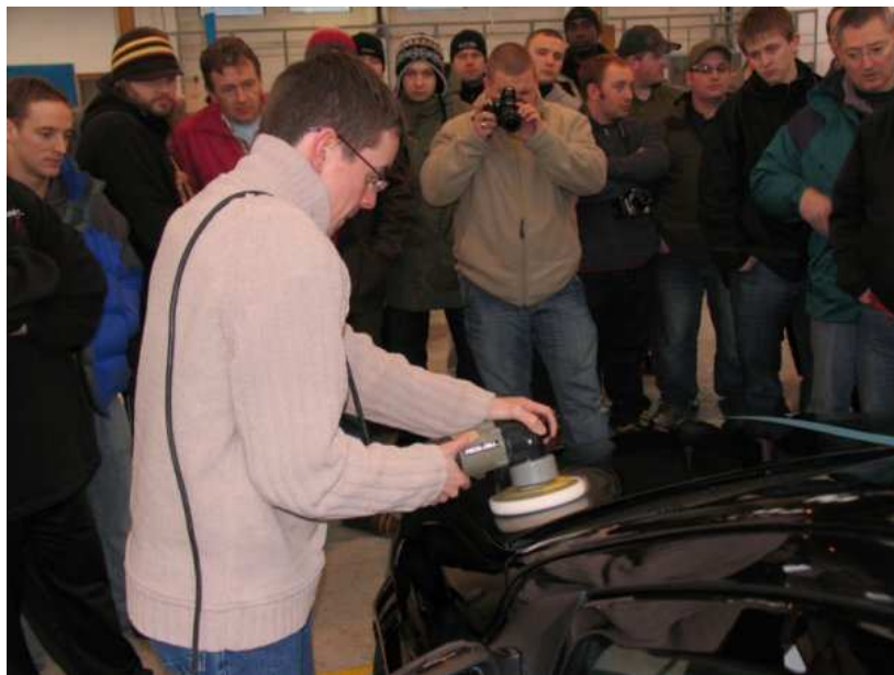
Typical hold for a Porter Cable 7424 Dual Action Polisher
