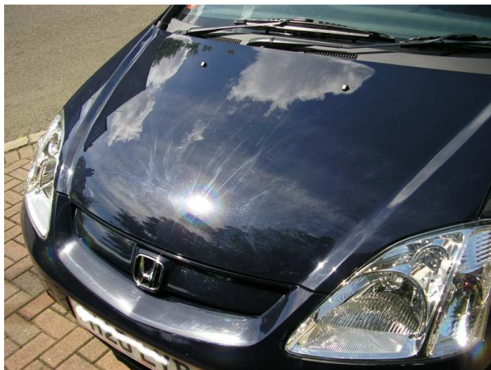
Holograms (from previous poorly finished machine polishing)
