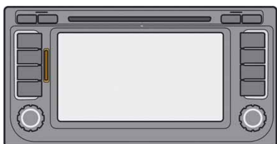
Front panel of RNS 510 with SD memory card reader in Touareg
