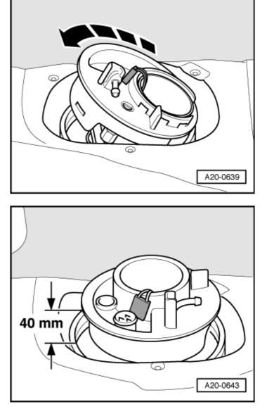
→ Hold flange in fitting position approx. 40 mm over opening.
