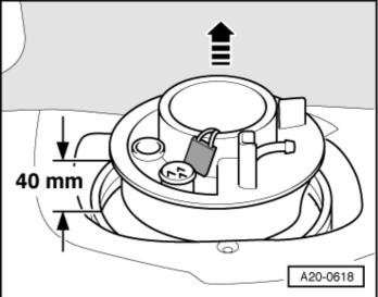
→ Remove flange seal from edge of opening.
