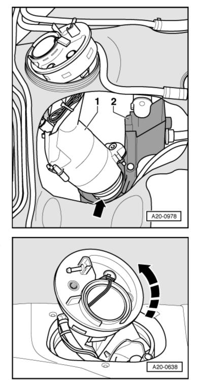
→ Now turn fuel delivery unit anti-clockwise 45°, which will lower the delivery unit into the fuel tank.
