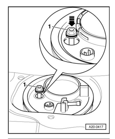
→ Pull the fuel delivery unit upwards approx. 40 mm while slightly turning side to side.
