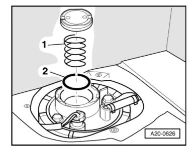
→ Using special tool 2012 A, carefully tighten flange for fuel gauge sender by turning it anti-clockwise as far as it will go.
