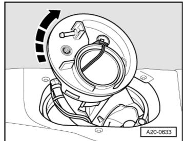
→ Now turn fuel delivery unit anti-clockwise 45° while pulling upwards...
