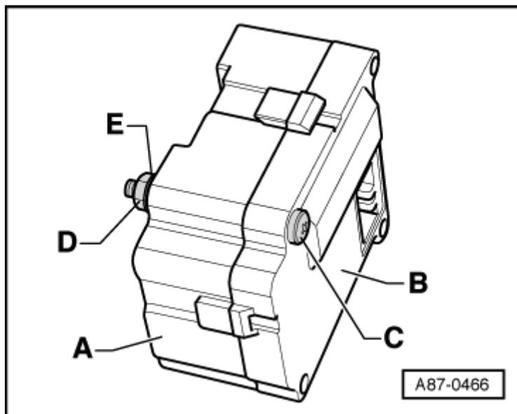
D- making contact with the air conditioner unit (the control motor is not bolted at this point).
