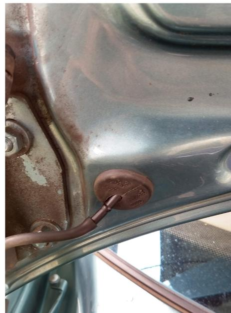
Pull this hose and block end whilst locking car with fob or key to prove you have a leaking actuator boot.
