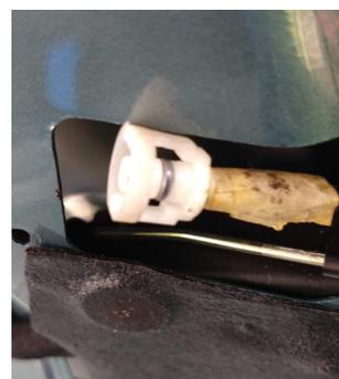
You will also have to remove this hose from the actuator before you remove it. Squeeze the sides of the white retaining thing and prise gently to release.
