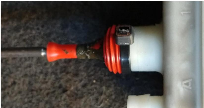
I added a ziplock tie and some gasket sealant as overkill, since I am installing a 26 year old part as a replacement!
