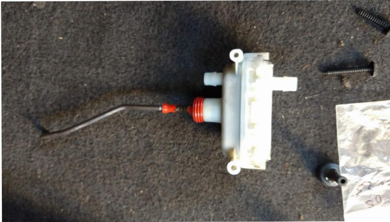
Slide the boot off the rod after prising it from the actuator housing.
