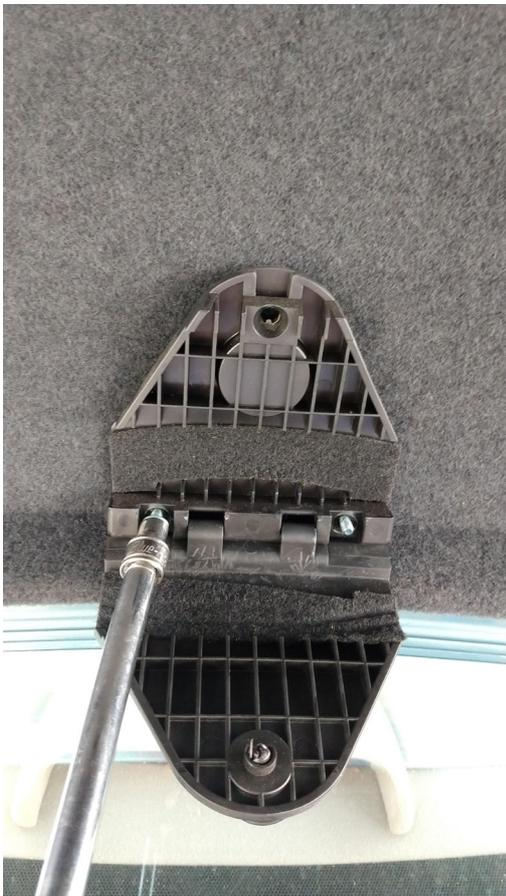
The safety triangle holder also has to be removed (10mm nut). There are two plastic trim clips that must be finessed from their locating holes. Probably be careful or they might break!
