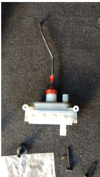
This is the vacuum pump lock actuator removed from the boot lid. It is held in by the two screws in the picture.
