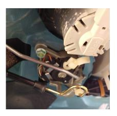
In my case the rod had somehow already come out of the mechanism without my intervention...! If you have the same case, there is a hole in the black part of the mechanism where it should be fitted as shown in the picture above.
