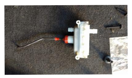
Slide the boot off the rod after prising it from the actuator housing.
