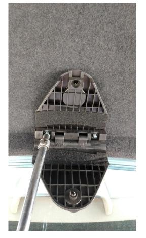
The safety triangle holder also has to be removed (10mm nut). The there are two plastic trim clips that must be finessed from their locating holes. Probably be careful or they might break!
