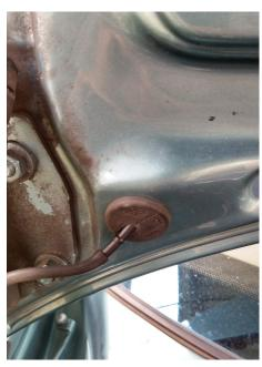
Pull this hose and block end whilst locking car with fob or key to prove you have a leaking actuator boot.
