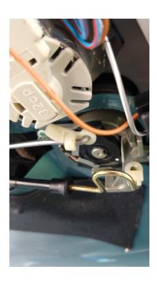
The silver rod has a whitish retaining clip securing it into the rear of the boot lid lock mechanism. Pull this clip away from the rod and you can then withdraw the rod downward and away from the mechanism. The other end of this rod is attached to the vacuum pump lock actuator.
