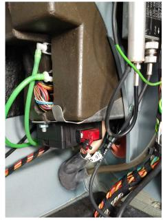
View of the central locking vacuum pump - located behind left boot compartment trim
