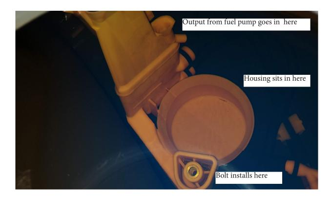
Here is what you must achieve to ensure the housing has been located correctly.
