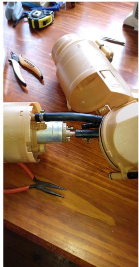
Bend the two retaining clips located on opposite sides of the fuel pump out of the way and the fuel pump can be withdrawn from the lower part of the housing by pulling on the hose attached to the pump spiggot. I found it to be a very tight fit so go easy, as you wouldn't want to break anything. Did i mention that already?
