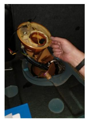
Eventually, the housing will be able to be lifted out of the tank. Have a bucket ready if the petrol tank wasn't empty!
